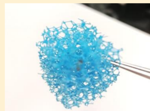
Fig. 2. A single element of the filter bed.
