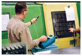
P-Trak Ultrafine Particle Counter and accessories includes: Telescoping Sample Probe, Shoulder Strap, Inlet Screen, Spare Wicks (2), Alkaline Batteries, Alcohol Fill Capsule with Storage Cap, Reagent Grade Isopropyl Alcohol, Zero Filters (2), Carrying Case, TrakPro®-Software, Computer Cable, Operation and Service Manual, Calibration Certificate, and Two-year Warranty.
